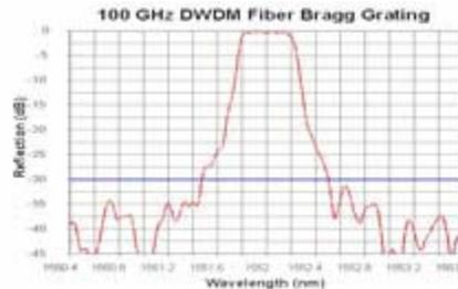
Figure 1: A typical 100GHz DWDM fiber Bragg grating reflective curve.
